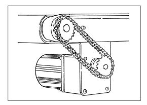
Remove the chain cover once every 6 months and apply grease to the chain using brush.
