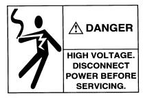
Make sure to cut off the breaker of controller while maintenance work is being done. Especially during such work for inside the box, disconnect connecting cable with molding machine and cut off primary power supply of the factory.
