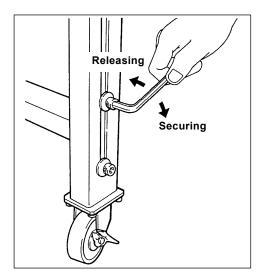
Loosen the height adjusting bolts (2 bolts  $\times$  4 to 6 places) located on each leg as shown in the illustration using a hexagon wrench and adjust the conveyer height.
