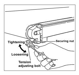
Adjust the belt tension using the tension adjusting bolts at both ends of conveying "IN" side if necessary.
