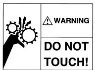
To work in moving zone for maintenance or other purposes, do not touch carelessly with such parts as motor, rotary axis, gear, pulley, belt which have danger of enfolding you. Cut off power supply and air pressure to work.
