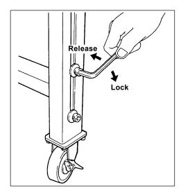
Use the hexagonal wrench to loosen the height adjustment bolts located on the stand legs near the casters (2 bolts  $\times$  4 positions), and adjust the height of the conveyer belt.
