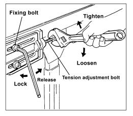
Adjust the belt tension only when the conveyer belt weaves or when the conveyer driving roller is rotating without transporting the belt. Otherwise, you do not need to adjust the belt tension.
