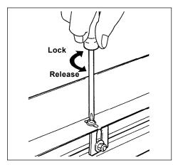
Loosen the installation bolt using a Philips screwdriver to adjust the width of the guide located on each side of the conveyer belt.
