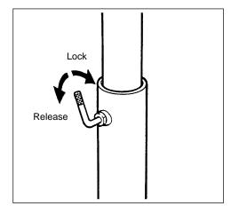
•Adjusting the slope angle
