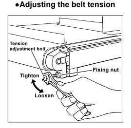
Adjust the belt tension only when the conveyer belt weaves or when the conveyer driving roller is rotating without transporting the belt.
