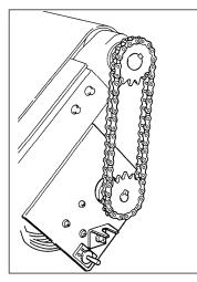
Remove the chain cover to apply grease to the chain once every six months.
