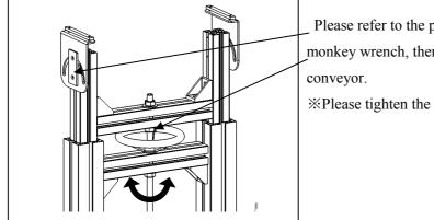
Please refer to the picture, first loosen the mounting nuts by a monkey wrench, then rotate the hand wheel to adjust the height of
