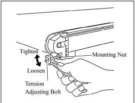
Adjust the belt tension by the tension adjusting bolts at both sides of move in side if necessary.
