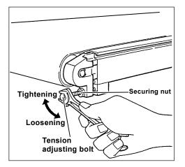
Adjust the belt tension using the tension adjusting bolts at both ends of conveying "IN" side if necessary.
