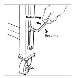
Loosen the height adjusting bolts (2 bolts × 4 to 6 places) located on each leg as shown in the illustration using a hexagon wrench and adjust the conveyer height. \* Note that after adjustment, tighten the bolts.
